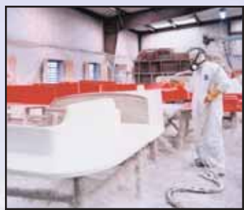
Chopped fiberglass being sprayed onto a gelcoated body mold.
