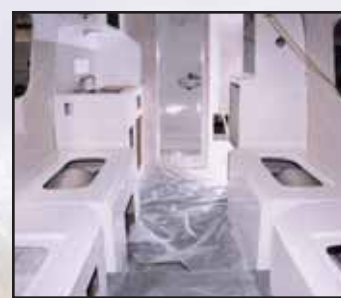
Lightweight liners for cabinets, seat bases & shower add strength & rigidity.
